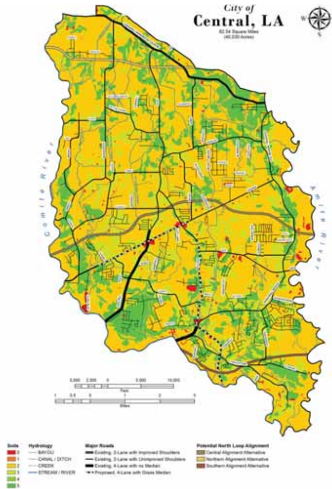
Soils were examined for their development capacity. Characteristics such as engineering bearing capacity and infiltration rates related to stormwater management were considered in the evaluation of twenty-one soils. In general, soils tested throughout the city rated primarily as moderate for development, with some isolated areas to the north and south rating as suitable.
